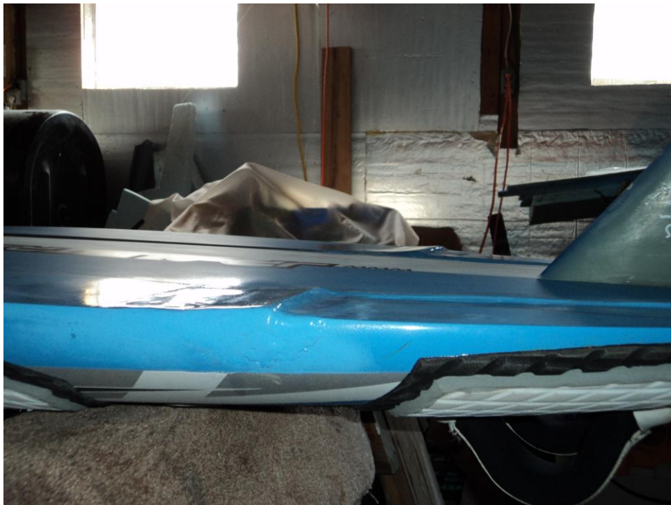
Figure 3 shows a side view of the Camber/slope step and the side step rounded cusp.
