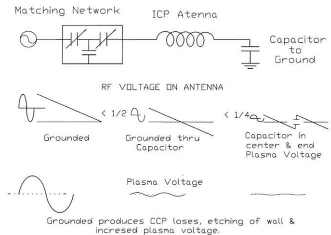
Fig 1 Driving an ICP, Antenna Voltages and Plasma Voltages
